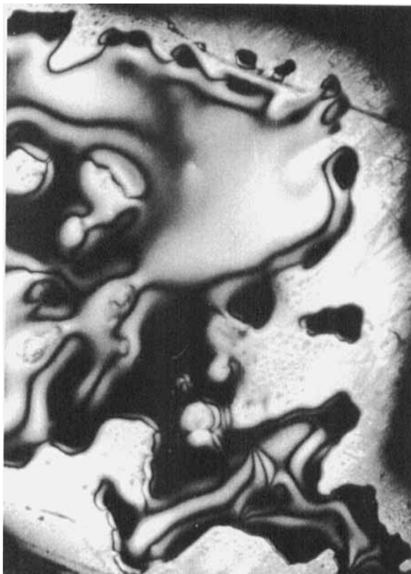
Figure 2. 11-INCu: T = 484 K; nematic schlieren texture. Crossed polarizers.
